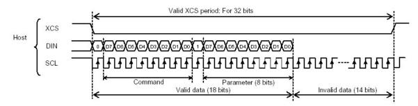
Note: In the above example, the 32-bit XCS signal is valid and fixed. This also applies to 16- or 24-bit applications.
