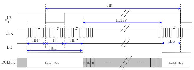
\*1. The frequency of CLK should be continued whether in display or blank region to ensure IC operating normally.
