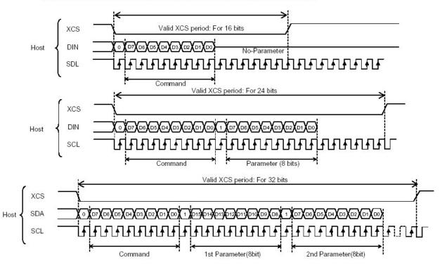
Example of introducing conventions for transferring the XCS signal in units of 8 bits
