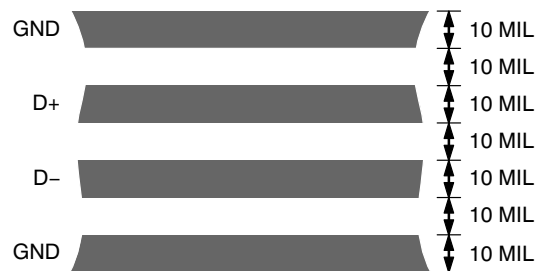
Figure 17. Arrangement of Signal Tracks
