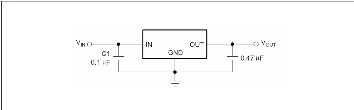
Figure 4. Application circuit for adjustable version
