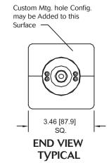
Units must be Mounted in such a way as to Allow for Free Air Flow Around fins to Assure Performance
