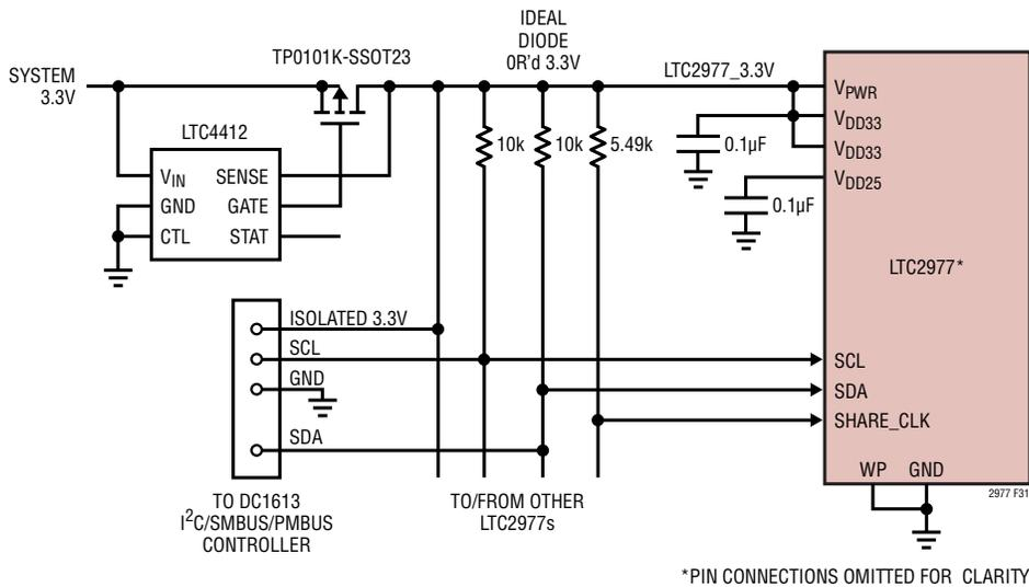
NOTE: DC1613 CONTROLLER I<sup>2</sup>C CONNECTIONS ARE OPTO-ISOLATED
