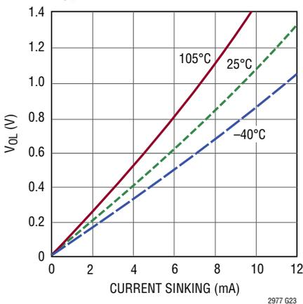
**V<sub>OUT\_EN[7:4]</sub> V<sub>OL</sub> vs Current**
