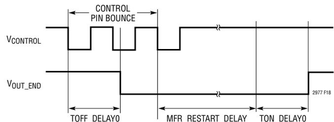
Figure 18. Off Sequence with Automatic Restart
