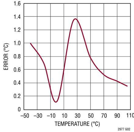
**ADC Total Unadjusted Error vs Temperature**
