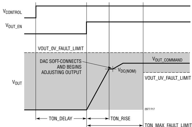
Figure 17. Typical On Sequence Using Control Pin
