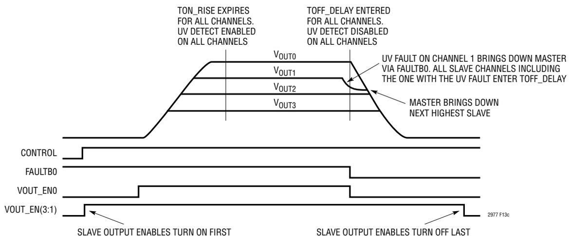
Figure 13c. Fault on Channel 1 Tracking All Supplies Down
