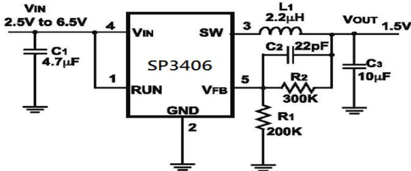
$$V_{out} = 0.6 \times \left(1 + \frac{R_2}{R_1}\right)$$
