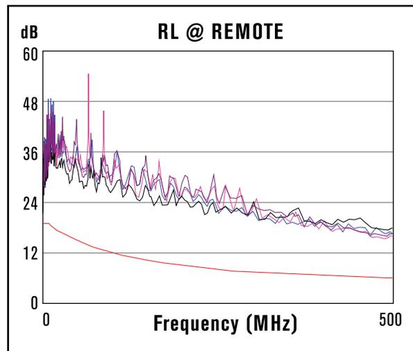
**Note:** Above graphs illustrate the main ethernet test results of the CarlisleIT Octax™ connectors and cable 26463/1A042X-8(LD). These charts were produced by using Fluke DTX 1800 test equipment with TIA/EIA-568 CAT 6A specification, 180 ft of cable, and 4 connectors. Drawings, test report, and other contact arrangements will be available upon request. Contacts are included with connector.
