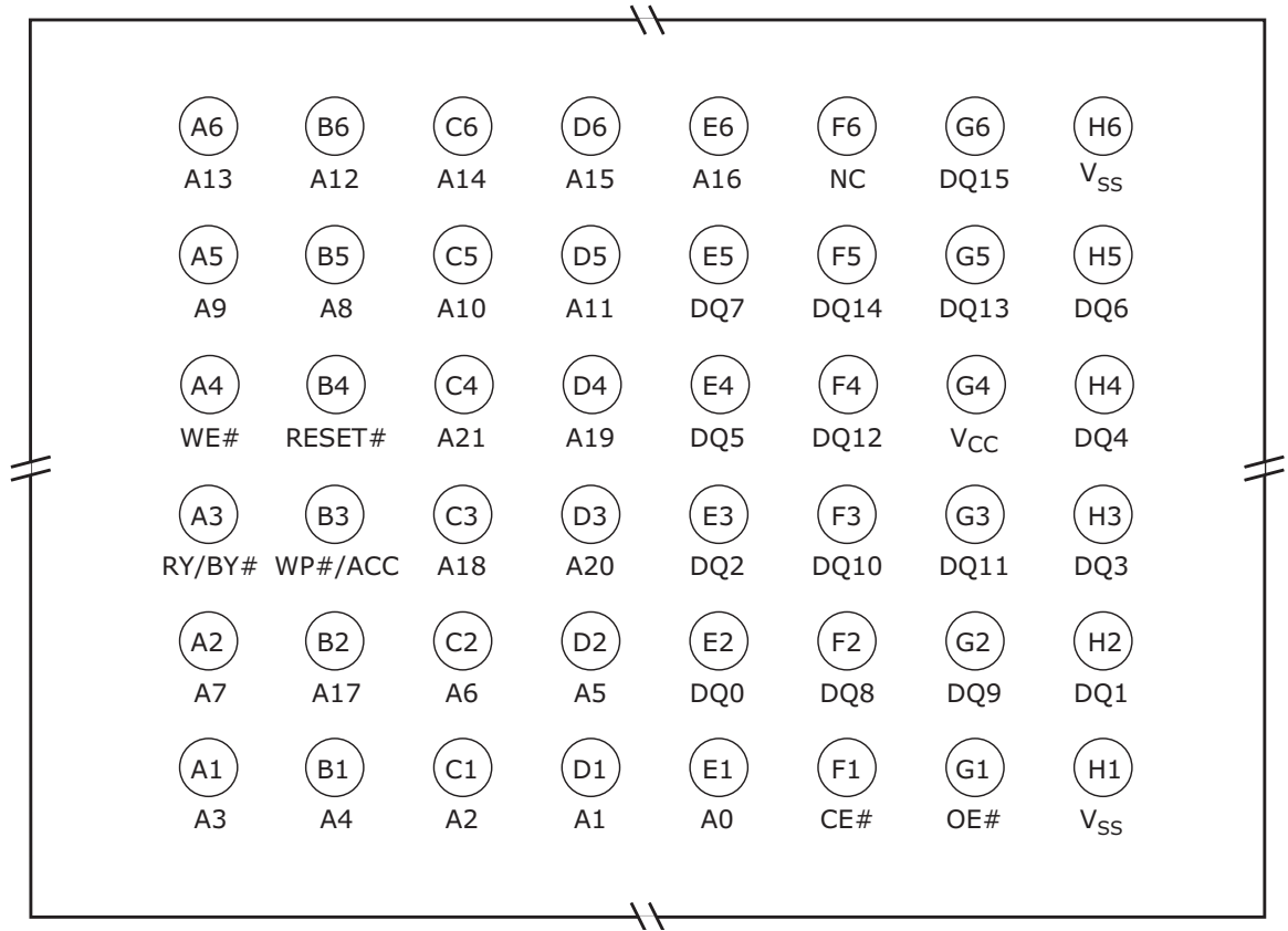
Figure 7.3 48-Ball Fine-Pitch BGA, Top View, Balls Facing Down—PL064J—PL032J: C4(A21)=NC
