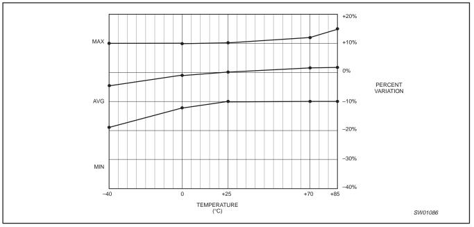
Figure 15. Typical frequency variation over process at  $V_{\text{DD}}$  = 3.0 V to 5.5 V
