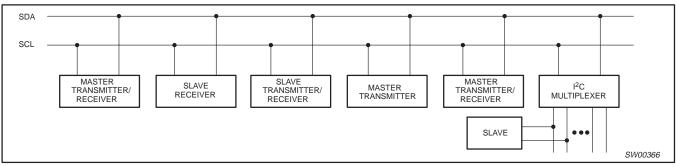
Figure 8. System configuration
