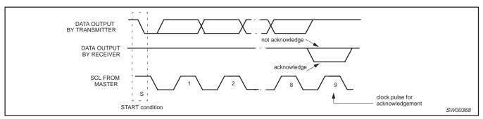
Figure 9. Acknowledgement on the I<sup>2</sup>C-bus
