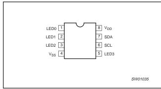
Figure 1. Pin configuration
