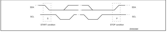
Figure 7. Definition of start and stop conditions
