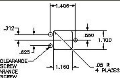
BOTTOM MOUNT-CLEARANCE HOLE FOR .192 SCREW
