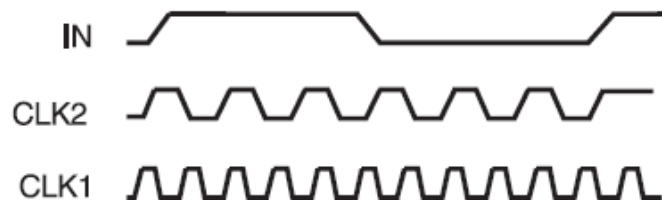
Input and Output Clock Waveforms with CLK2 Connected to FBIN
