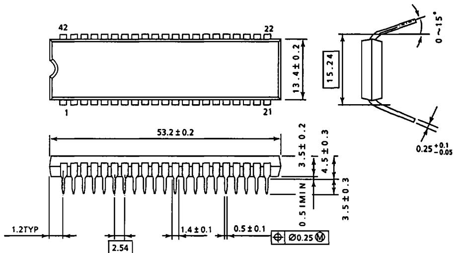
Note : Package width and length do not include mold protrusion, allowable mold protrusion is 0.15mm.
