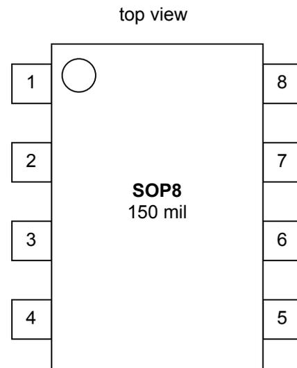
Fig. 3: Pin Configuration
