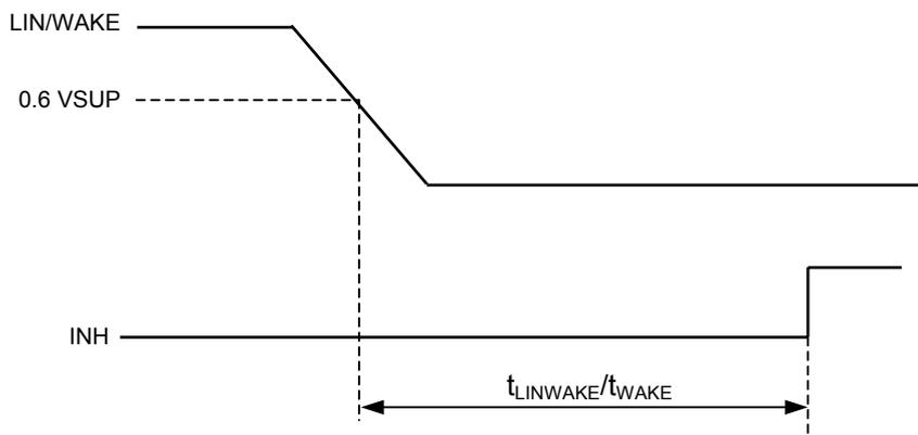
Figure 6: Bus Wake Up and WAKE Timing Description
