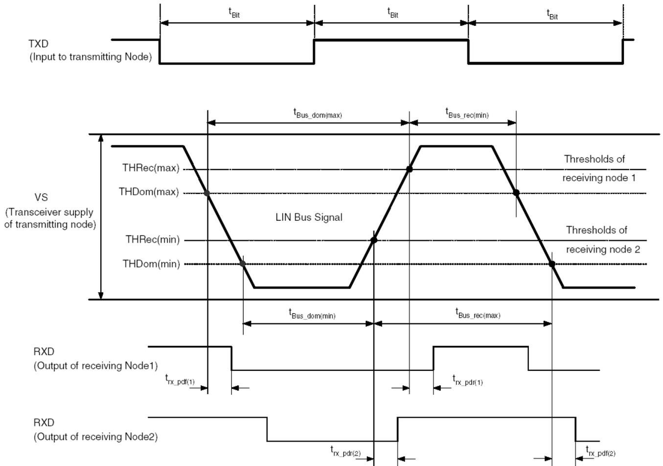
Fig. 5: LIN Bus Driver Timing Characteristics
