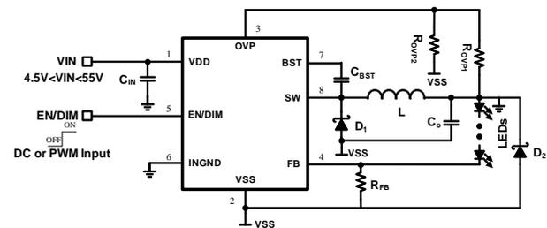
**Figure 2: Buck-Boost Application where LED+ Possibly Shorted to VSS**
