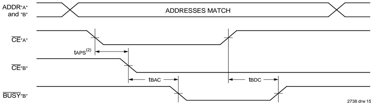
Waveform of **BUSY** Arbitration Cycle Controlled by Address Match Timing<sup>(1)</sup> ( $M/\bar{S} = V_{IH}$ )
