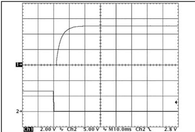
**Figure 9:** Turn-on transient at full load (resistive load) (10 ms/div). Input voltage pre-applied. Ch 1: V<sub>out</sub> (2V/div) Ch 2: ON/OFF input (5V/div)
