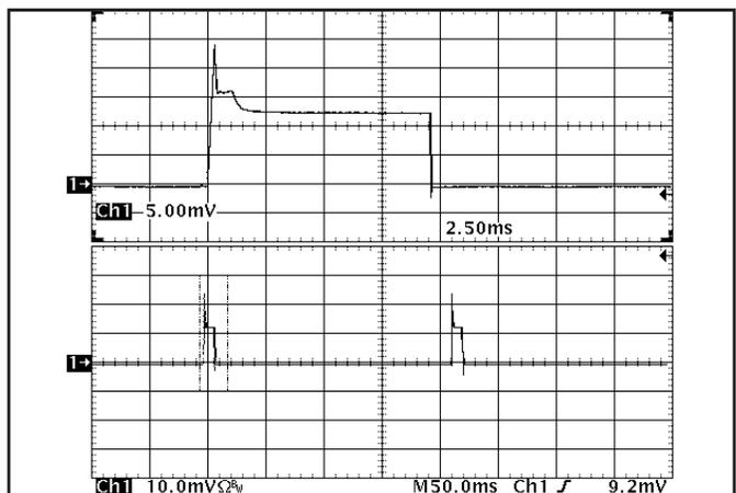
**Figure 18:** Load current (5A/div) as a function of time when the converter attempts to turn on into a  $10\ \text{m}\Omega$  short circuit. Top trace (2.5ms/div) is an expansion of the on-time portion of the bottom trace.
