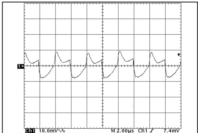
**Figure 16:** Output voltage ripple at nominal input voltage and rated load current (20 mV/div). Load capacitance:  $1\ \mu\text{F}$  ceramic capacitor and  $10\ \mu\text{F}$  tantalum capacitor. Bandwidth: 20 MHz. See Figure 13.
