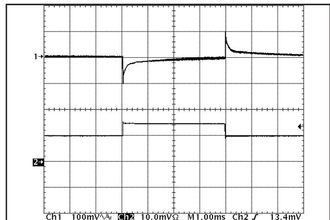
**Figure 12:** Output voltage response to step-change in load current (50%-75%-50% of I<sub>out</sub>(max); dI/dt = 5A/μs). Load cap: 470μF, 30 mΩ ESR tantalum capacitor and 1μF ceramic cap. Ch 1: V<sub>out</sub> (100mV/div), Ch 2: I<sub>out</sub> (5A/div).
