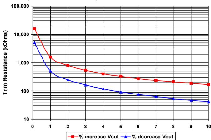
Figure C: Trim Graph for 5.0V<sub>out</sub> module
