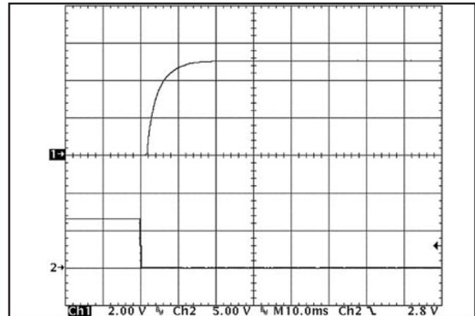
**Figure 10:** Turn-on transient at zero load (10 ms/div). Ch 1: V<sub>out</sub> (2V/div) Ch 2: ON/OFF input (5V/div)
