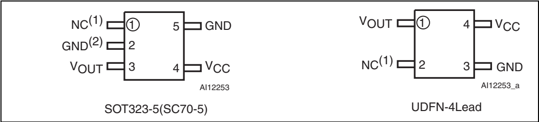
Figure 2. Connections (top view)
