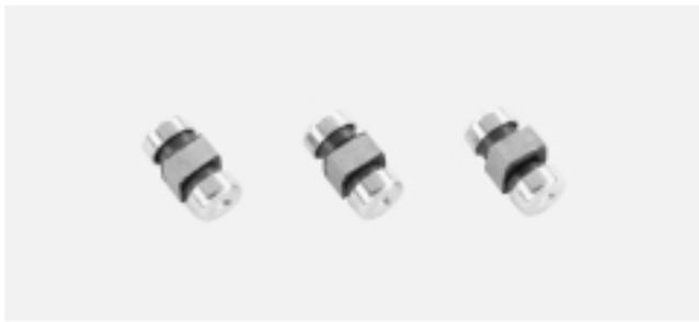
The NFM60R Series is an EIA standard 1206 size version of the NFM61R. Its high rated current (6A) and low voltage drop due to small DC resistance (Typ. 3 ~ 4mΩ) are suitable for DC power line use. The feedthrough capacitor provides excellent high-frequency characteristics. The series has excellent solder heat resistance. Both flow and reflow soldering method can be employed. (Only reflow soldering should be employed with the NFM60R20T152.)
