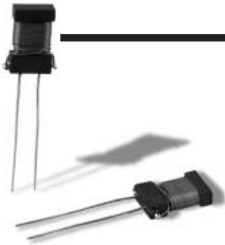
The RL-1170 is an economical inductor with a unique flat coil configuration that makes it ideally suited for use in high density and high frequency printed circuit board assemblies with current ratings from 27mA to 2.25A. Inductance values 1.0 $\mu$ H to 4.7MH with 45 values to choose from. Its vertical design is unique and space-saving.
