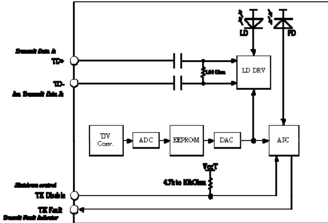
LD DRV: Laser diode driver, DAC: Digital to analogue converter, T/V Conv.: Temperature to voltage converter, APC: Automatic power control circuit, ADC: Analogue to digital converter, EEPROM: Electronic erasable ROM, PD: Photo Diode, LD: LASER Diode
