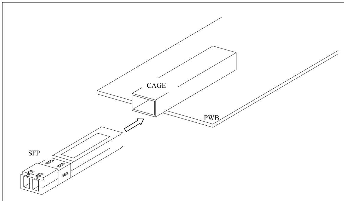
**Fig.** Insert direction
