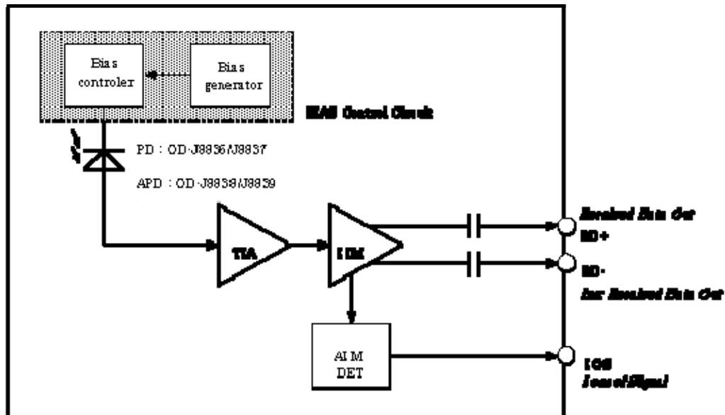
APD: Avalanche Photo Diode, TIA: Trans Impedance Amplifier, LIM: Limiting amplifier, ALM DET: alarm detector
