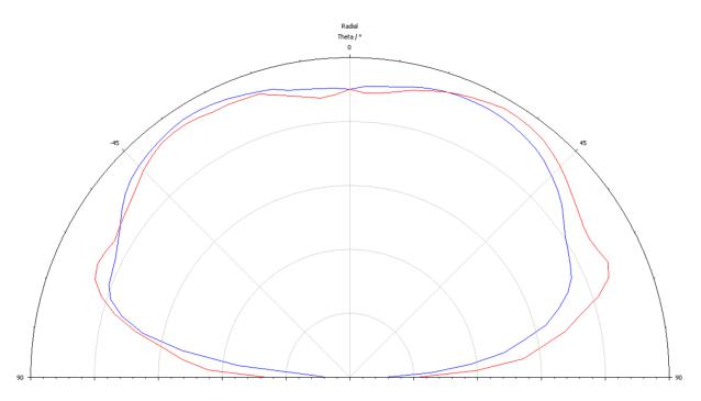
This is a representative radiation pattern for the TR5270 (250-µm) LED product. Actual patterns will vary slightly for each chip.
