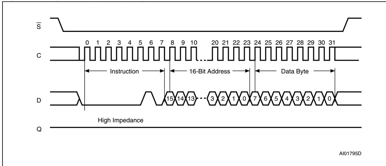
1. Depending on the memory size, as shown in [Table 5](#), the most significant address bits are Don't Care.
