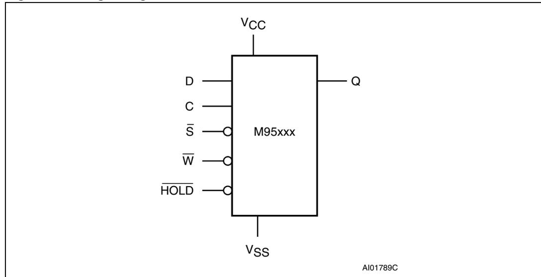
The SPI bus signals are C, D and Q, as shown in [Figure 1](#) and [Table 1](#). The device is selected when Chip Select ( $\overline{S}$ ) is driven low. Communications with the device can be interrupted when the  $\overline{HOLD}$  is driven low.
