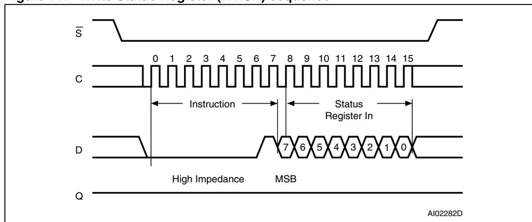
Driving the Chip Select ( $\bar{S}$ ) signal high at a byte boundary of the input data triggers the self-timed Write cycle that takes  $t_{wv}$  to complete (as specified in AC tables under [Section 9: DC and AC parameters](#)).
