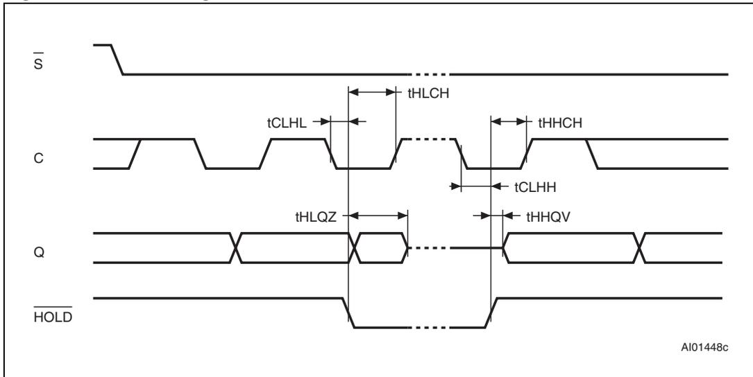
Figure 22. Serial output timing
