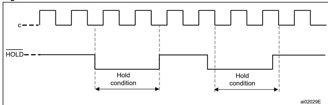
The Hold condition starts when the Hold ( $\overline{HOLD}$ ) signal is driven low when Serial Clock (C) is already low (as shown in [Figure 7](#)).
