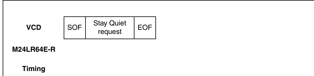
Figure 53. Stay Quiet frame exchange between VCD and M24LR64E-R
