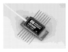
The LSC26xx also has 30 dB of optical isolation which is temperature controlled to maintain isolation over the full operating temperature range.
