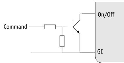
By releasing the On/Off function, the converter will restart within the start-up time specifications given in table page 3. For further details please consult "Logic On/Off" application note.
