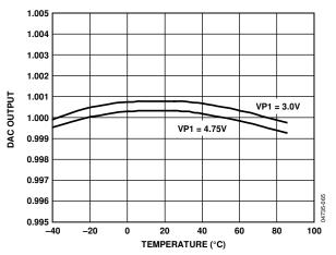
Figure 19. DAC Output vs. Temperature
