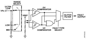
Figure 22. Supply Fault Detector Block
