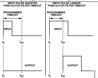
Figure 23. Input Glitch Filter Function
