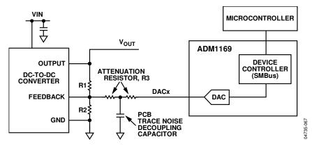
Figure 32. Open-Loop Margining System Using the ADM1169
