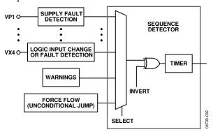
Figure 27. Sequence Detector Block Diagram
