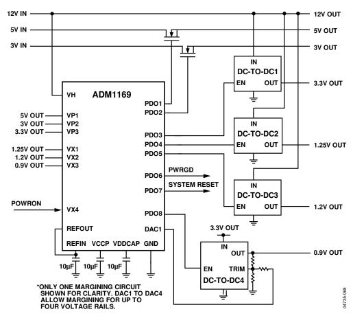
Figure 34. Applications Diagram
