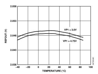
Figure 20. REFOUT vs. Temperature
