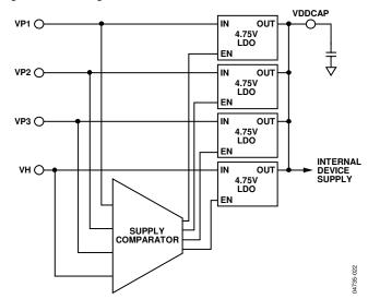
Figure 21. V<sub>DD</sub> Arbitrator Operation
