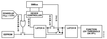
Figure 35. Configuration Update Flow Diagram
