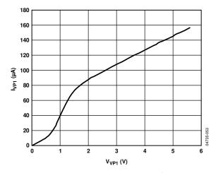
Figure 8. I<sub>VP1</sub> vs. V<sub>VP1</sub> (VP1 Not as Supply)
