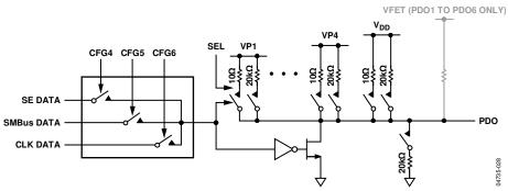
Figure 25. Programmable Driver Output
