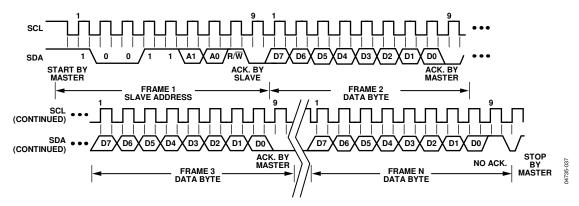
Figure 37. General SMBus Read Timing Diagram
