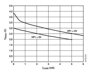
Figure 12. V<sub>PDO1</sub> (Strong Pull-Up to VPx) vs. I<sub>LOAD</sub>
