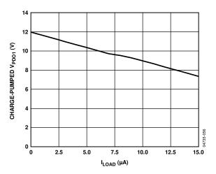
Figure 11. Charge-Pumped V<sub>PDO1</sub> (FET Drive Mode) vs. I<sub>LOAD</sub>
