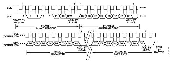
Figure 36. General SMBus Write Timing Diagram
