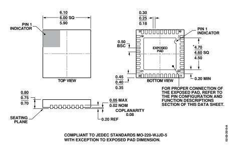
Figure 49. 40-Lead Lead Frame Chip Scale Package [LFCSP\_WQ] 6 mm × 6 mm Body, Very Thin Quad (CP-40-7) Dimensions shown in millimeters
