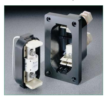
Littelfuse compact LTFD Series holders are designed for use as a combination fuseholder and disconnect switch for telecommunications equipment. The rugged unit utilizes a pull-out fuse carrier to safely disconnect power and provide easy fuse replacement.
