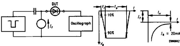
Pulse generator:  $t_p = 5\text{ }\mu\text{s}$ ,  $D = 0.05$
