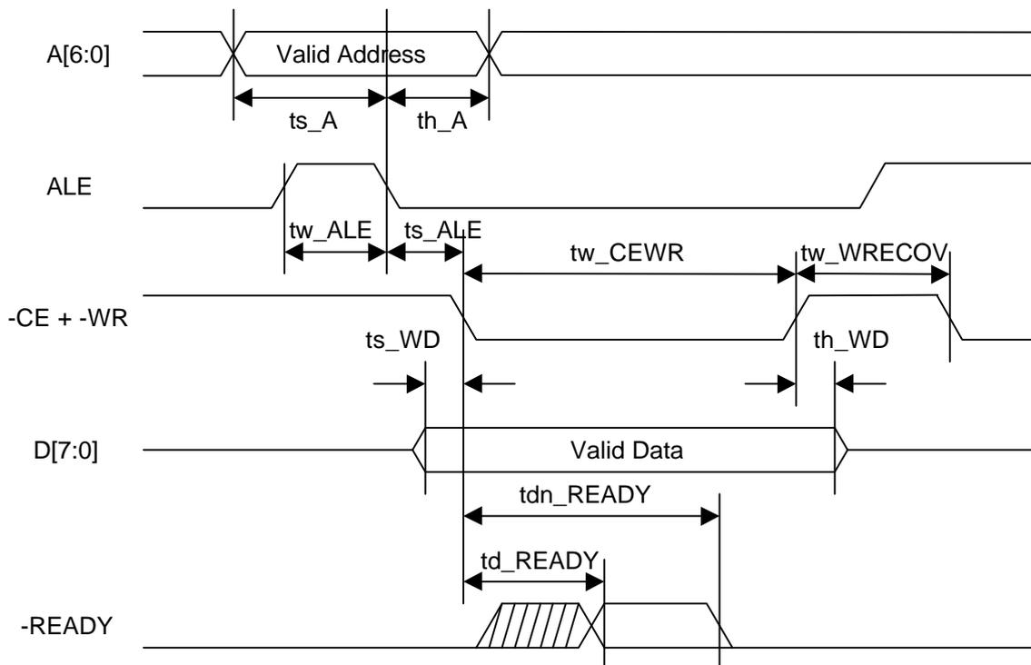
Figure 9.3.3 CPU Interface Write Access with Active ALE
