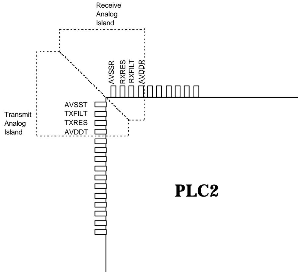
1. Resistors and capacitors connected to RXRES or RXFILT should be included in receive analog island.
