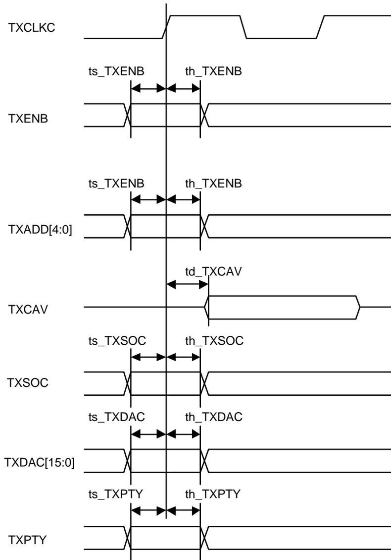
Fig. 9.2.1 TX Cell Interface Timing
