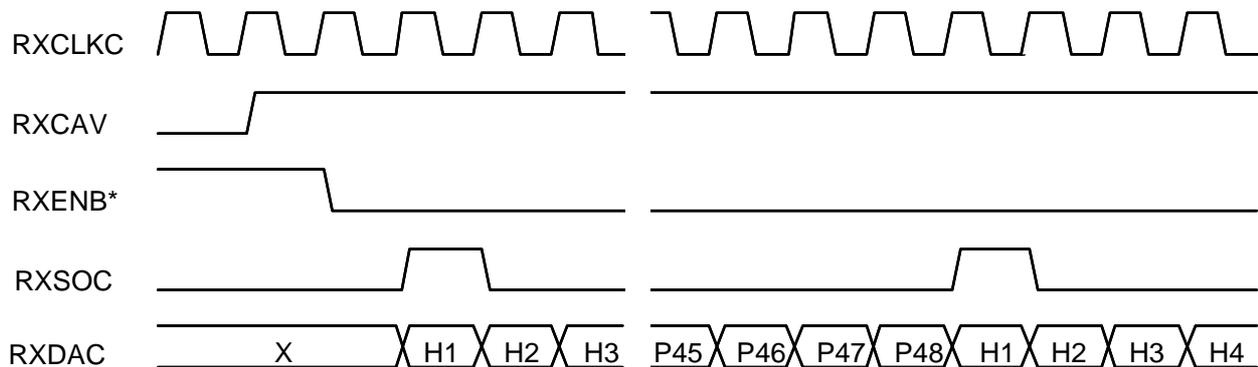
Figure 2.4.5 Receive Cell Transfer (1)
