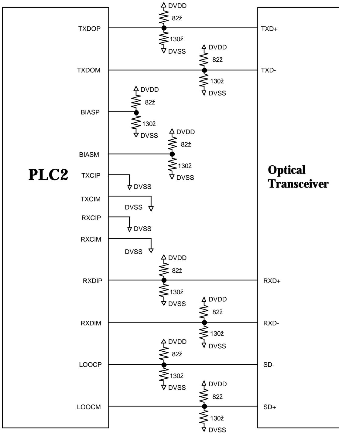
It is assumed that SD is asserted high when certain level of optical signal is detected. If SD output of the optical transceiver has single ended, meaning that only SD+ is output, then LOOCP input should be tied to 3.7V. It is realized, for instance, by tying LOOCP to DVDD via 1.3KΩ and to DVSS via 3.7kΩ.
