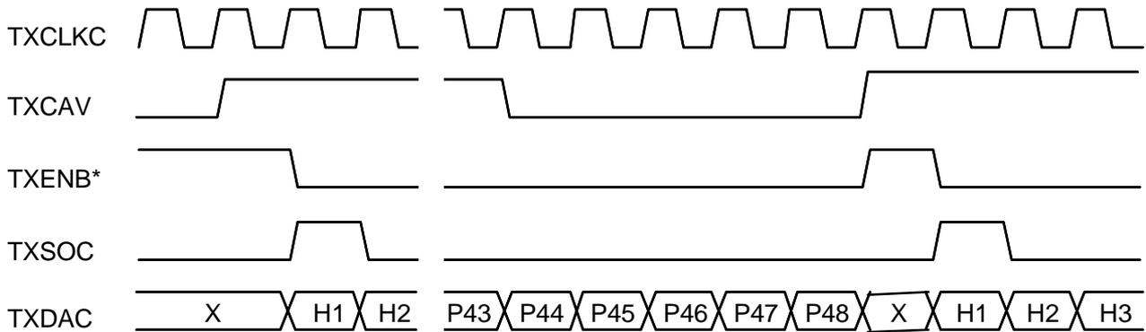
Figure 2.4.4 Transmit Cell Transfer (4)
