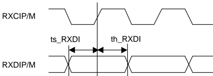
Figure 2.3.1 RX Line Interface Timing
