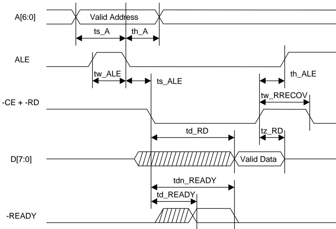
Figure 2.5.1 Host CPU Read Access Timing with Active ALE
