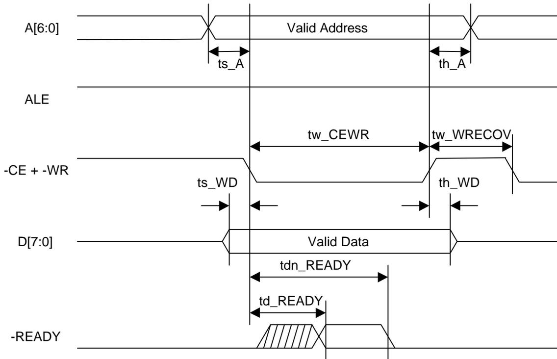
Figure 9.3.4 CPU Interface Write Access with Fixed ALE
