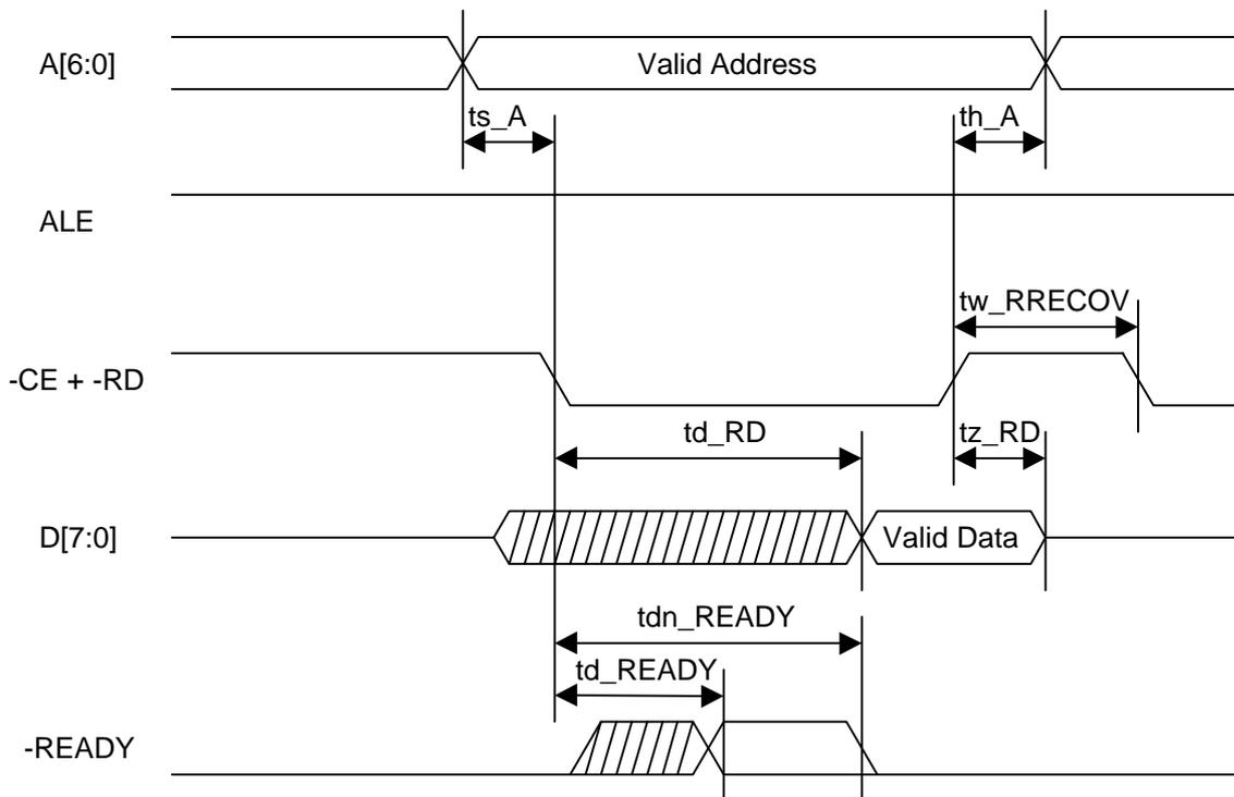
Figure 9.3.2 CPU Interface Read Access with Fixed ALE
