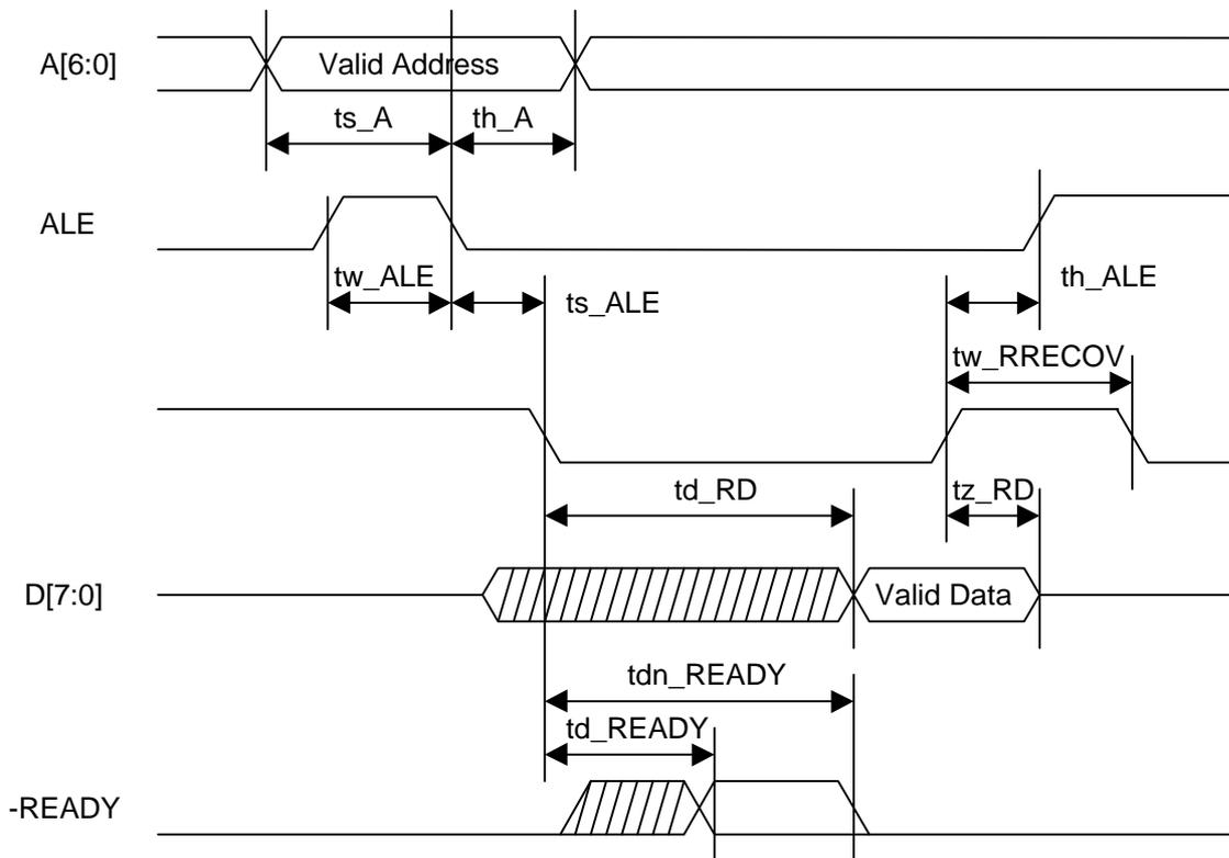
Figure 9.3.1 CPU Interface Read Access with Active ALE
