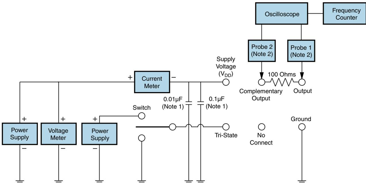
Note 1: An external  $0.01\mu F$  ceramic bypass capacitor in parallel with a  $0.1\mu F$  high frequency ceramic bypass capacitor close (less than 2mm) to the package ground and supply voltage pin is required.
