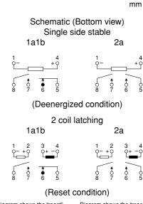
Diagram shows the "reset" position when terminals 3 and 4 are energized. Energize terminals 1 and 2 to transfer contacts. Diagram shows the "reset" position when terminals 3 and 4 are energized. Energize terminals 1 and 2 to transfer contacts.
