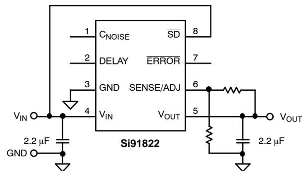
FIGURE 2. Adjustable Output
