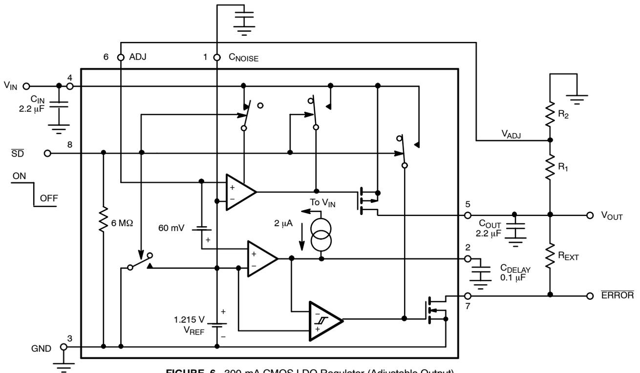
**FIGURE 6. 300-mA CMOS LDO Regulator (Adjustable Output)**
