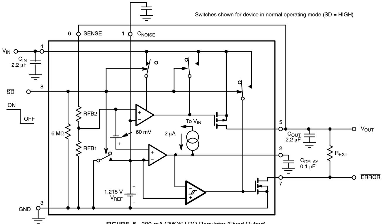
**FIGURE 5. 300-mA CMOS LDO Regulator (Fixed Output)**
