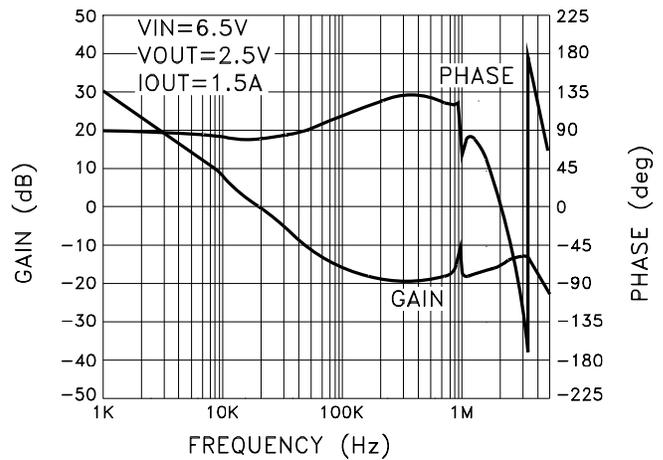
MSK5922-2.5RH GAIN AND PHASE vs. FREQUENCY
