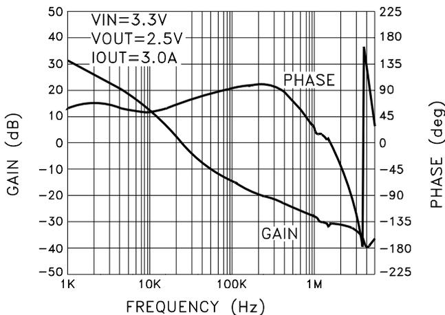
MSK5922-2.5RH GAIN AND PHASE vs. FREQUENCY
