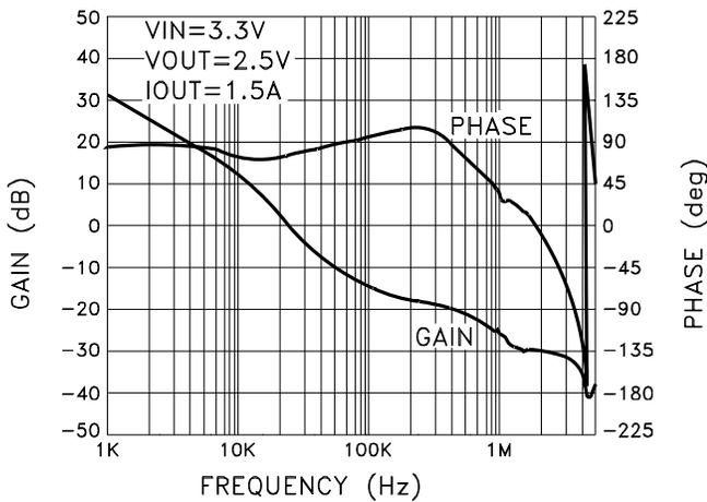
MSK5922-2.5RH GAIN AND PHASE vs. FREQUENCY
