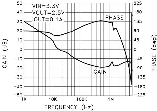
MSK5922-2.5RH GAIN AND PHASE vs. FREQUENCY
