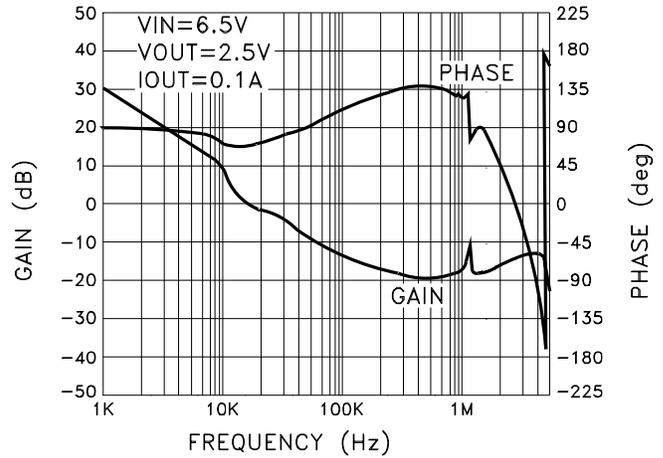
MSK5922-2.5RH GAIN AND PHASE vs. FREQUENCY
