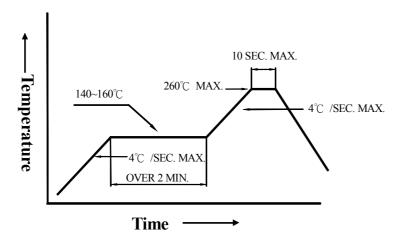
3. DIP soldering (Wave Soldering):
