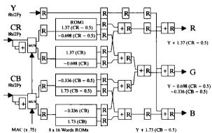
The R, G, B signal can be delayed by 1 Clock Period at the output of the matrix operator using the O/E F external command in order to allow frame interleaving in staggered rows.
