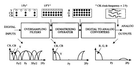
In order to be compatible with CCIR 601 all filters must have a linear phase and a flat response within the frequency band (5.5 MHz for Y and 2 MHz for CR and
