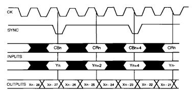
All internal registers are clocked on the falling edge of CK clock. Internal data paths have been scaled to allow output data in the range [0,255/256] for R, G, B and input data in the range [00, FF] for Y, CR, CB. Saturation circuits are used for out of range data, rounding functions are performed before truncation.
