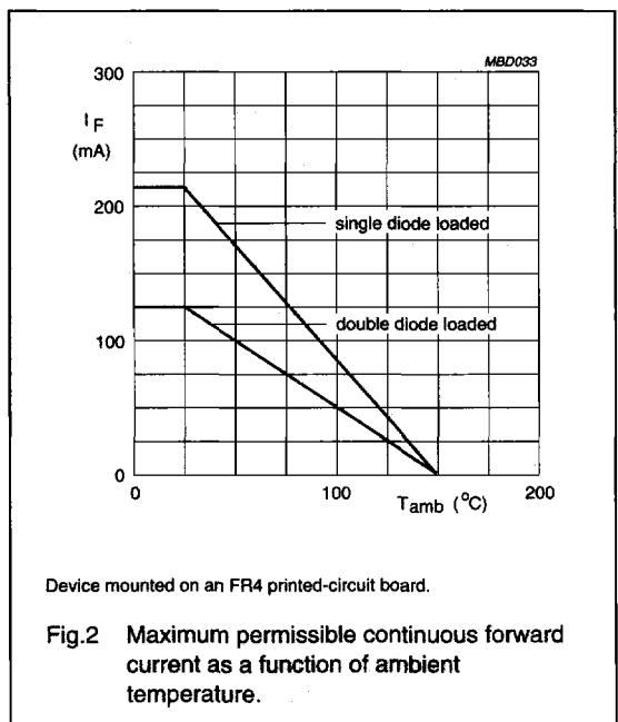
Fig.2 Maximum permissible continuous forward current as a function of ambient temperature.
