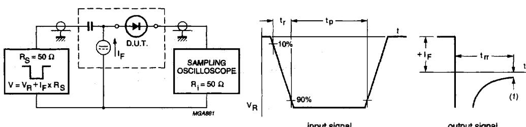
Fig.7 Reverse recovery voltage test circuit and waveforms.
