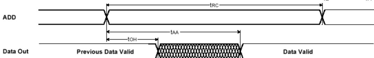
FIGURE 4. TIMING WAVEFORM OF READ CYCLE<sup>(2)</sup> ( $\overline{WE} = V_{IH}$ )
