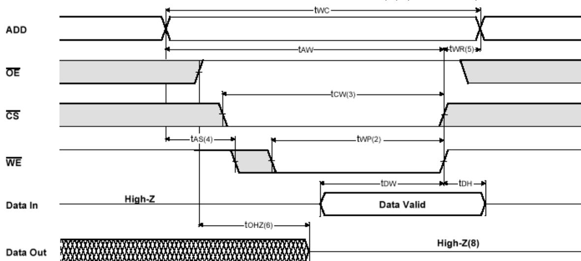
FIGURE 2. TIMING WAVEFORM OF WRITE CYCLE ( $\overline{OE}$  LOW FIXED)
