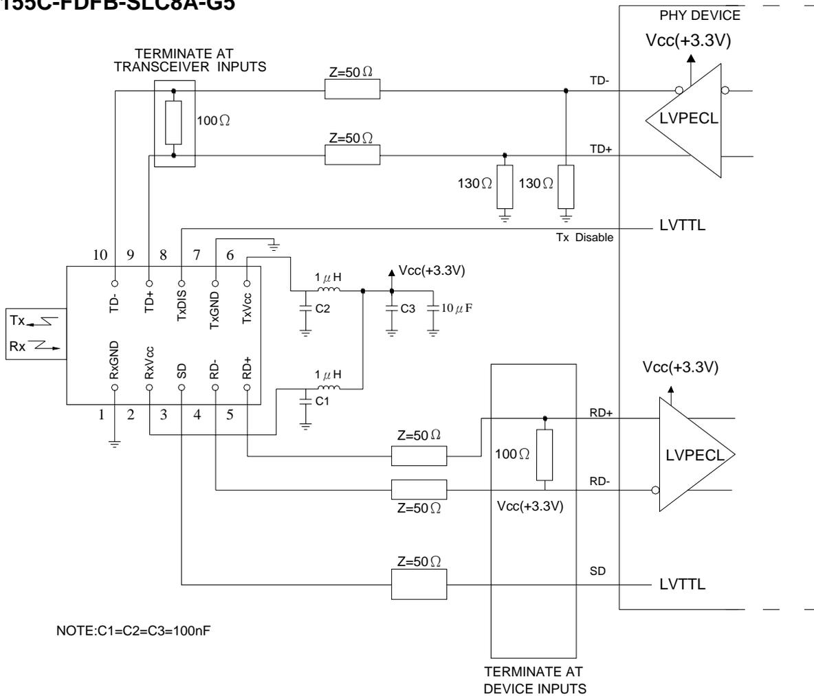
The split-loaded terminations for ECL signals need to be located at the input of devices receiving those ECL signals.
