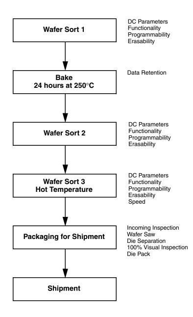
Figure 1. AMD KGD Product Test Flow
