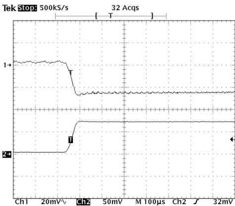
Operating conditions are as follows:  $V_{in}=5V$ ,  $V_o=3.3V$ , Load change from  $I_o=100\%$  to  $I_o=0\%$ ,  $T_A=25^\circ C$ ,  $C_{in}=0F$ ,  $C_o=\mu F$ .
