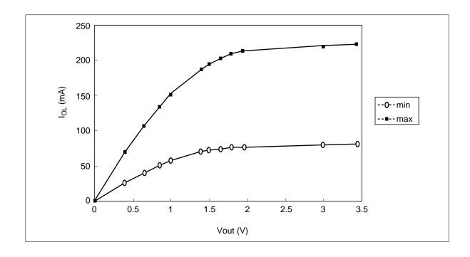
Output High Current ( $I_{OH}$ ) (Ta=0 to 65°C,  $V_{CC}=3.0~V$  to 3.45 V,  $V_{SS}=0~V$ )
