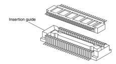
3) The connector has a simple lock mechanism.
