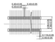
Recommended metal mask pattern Metal mask thickness: Here, 150 μm (Opening area ratio: 32 %)
