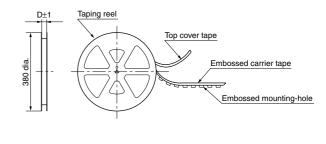
• Plastic reel dimensions (Conforming to EIAJ ET-7200B)
