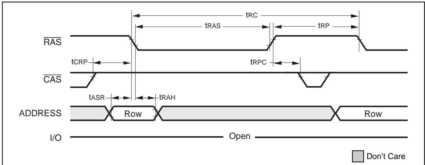
**$\overline{\text{CB}}\overline{\text{R}}$  REFRESH CYCLE** (Addresses;  $\overline{\text{WE}}$ ,  $\overline{\text{OE}}$  = DON'T CARE)
