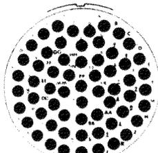
Arrangements are shown looking at pin face (socket is opposite). Cavity identifying letters or numbers are for reference only. Actual marking shall be as required by applicable specifications.
