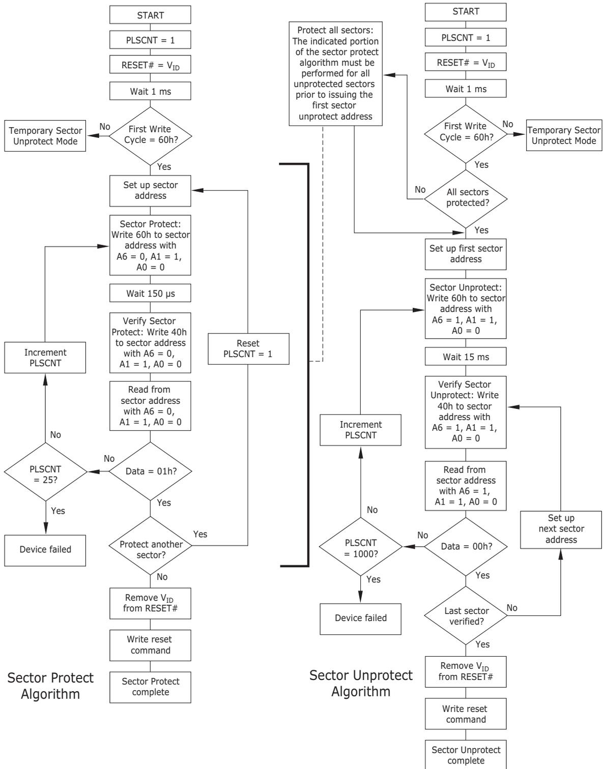
Figure 2. In-System Sector Protect/Unprotect Algorithms
