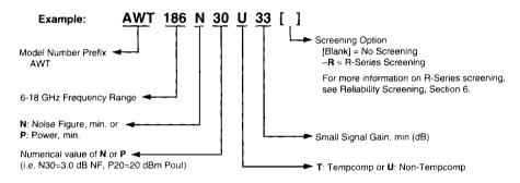
This example would order a 6–18 GHz amplifier with a noise figure of 3.0 dB max, no temp comp, a small signal gain of 33 dB minimum, and NO "R" Series Screening.
