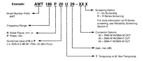
This example with a ~40R suffix would order a 6–18 GHz amplifier with a Pout of 20 dBm minimum, no temp comp, a small signal gain of 29 dB minimum, a SMA-male input connector and SMA-female output connector, and "R" Series Screening.
