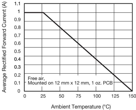
Fig. 1 - Derating Curve for Output Rectified Current
