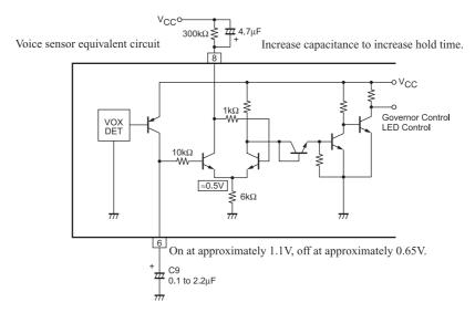
5. In record mode, grounding pin 8 will turn off the voice sensor circuit and keep the motor drive circuit operating continuously.
