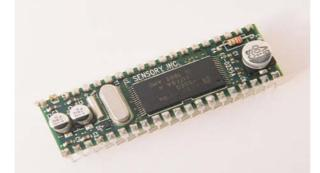
memory, Sensory's entire FluentChip<sup>™</sup> library can be utilized including Record and Playback, along with lots of extended speech. The RPM is a prototyping tool designed for developers who will be creating product system designs that feature RSC-4x processor chips.
