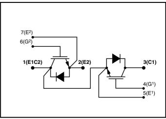
Fig. 1 Half bridge circuit diagram
